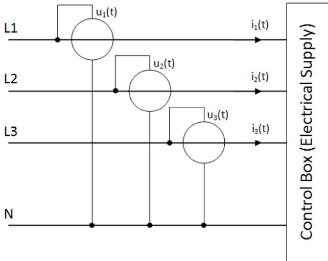
Fig. 1 Measurement setup for heat emissions from machines
