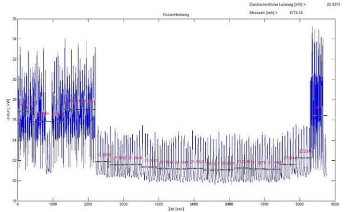
Fig. 6 measurements of a laser cutting-off machine within 3 hours
