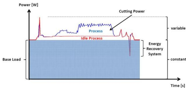
Fig. 2 Example of power use behavior of a specific machine over time
