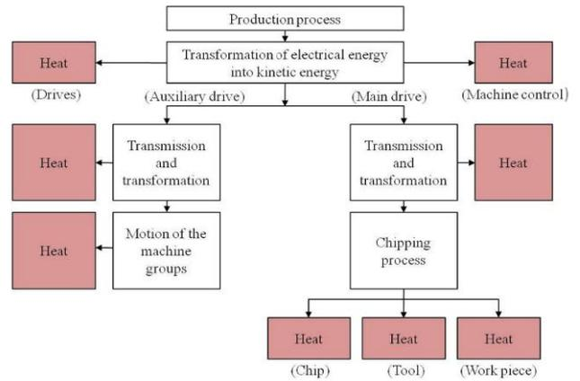
Fig. 3 Thermal transformation of machine components (Gleich 2008)
