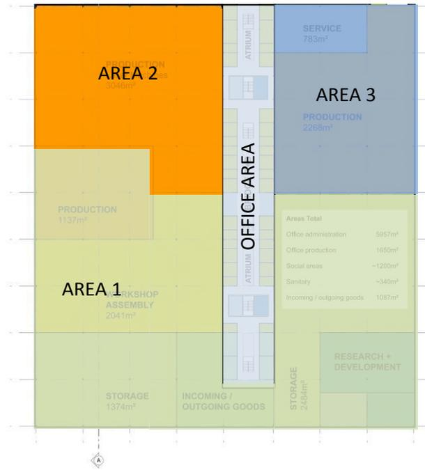
Fig. 10 Plan of the industrial facility
