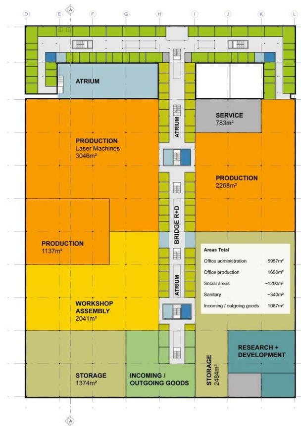
Fig. 8 Floor layout in the new facility design
