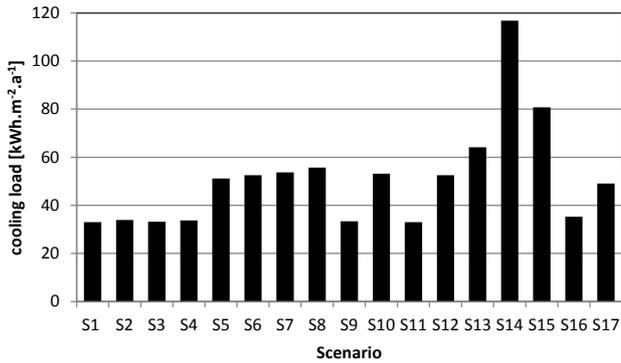
Fig. 11 Simulated annual cooling load (area 1-3) for all scenarios [ $\text{kWh}\cdot\text{m}^{-2}\cdot\text{a}^{-1}$ ]
