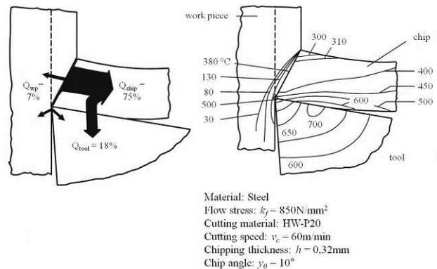
Fig. 4 Thermal behavior of the cutting process (Tönshoff and Denkena 2003)
